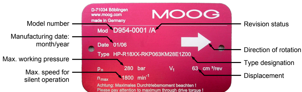
Figure 6: Nameplate of the RKP-II
